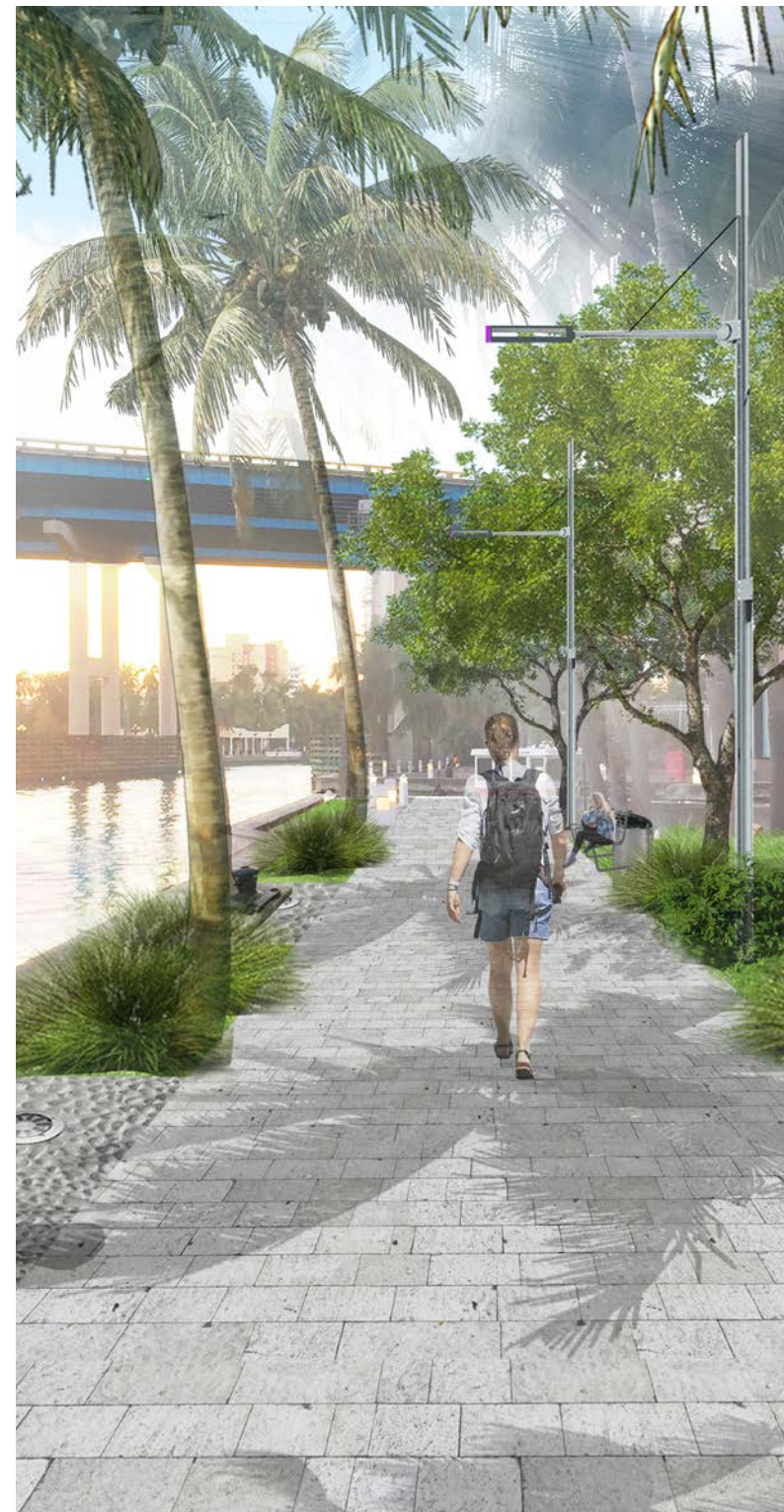
Concrete pavers give the Miami Baywalk & Riverwalk a unified, but distinct character. They are also easy to maintain and replace. LEFT: Miami Riverside Center heading to SW 1st Ave Bridge. RIGHT: Bayfront Park heading to Bayside Marketplace.
